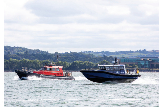
// Pioneer is a 100% electric foiling pilot vessel
