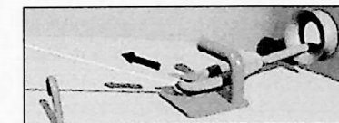
Heaving line from tug line disconnected from fixing-hook to windlass
