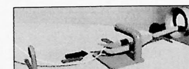
Slack the heaving line and the tug line is connected to the Safety Bitt
