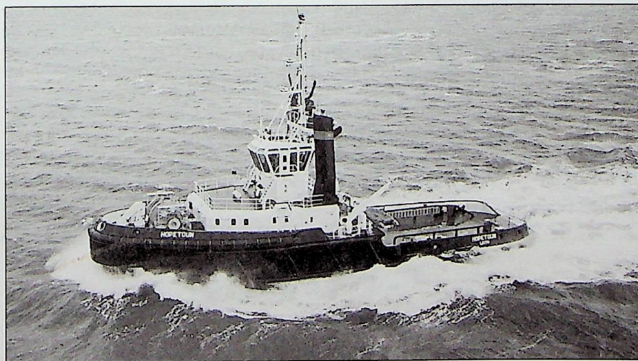
Hopetoun, 125 tons bollard pull, the most powerful escort tug in the UK.
