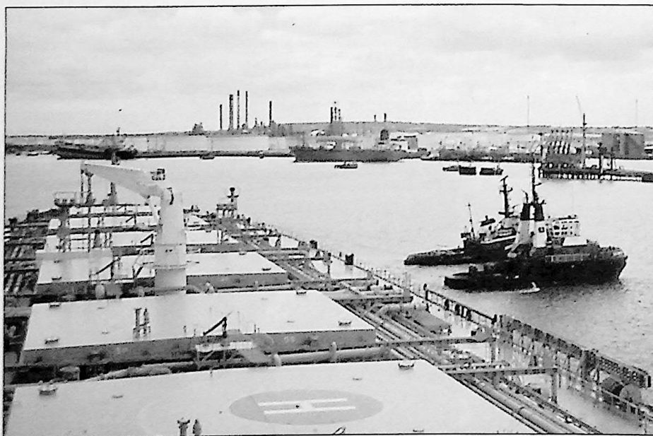
Swinging large vessels 180° in restricted waterways requires precise positioning and speed control.
