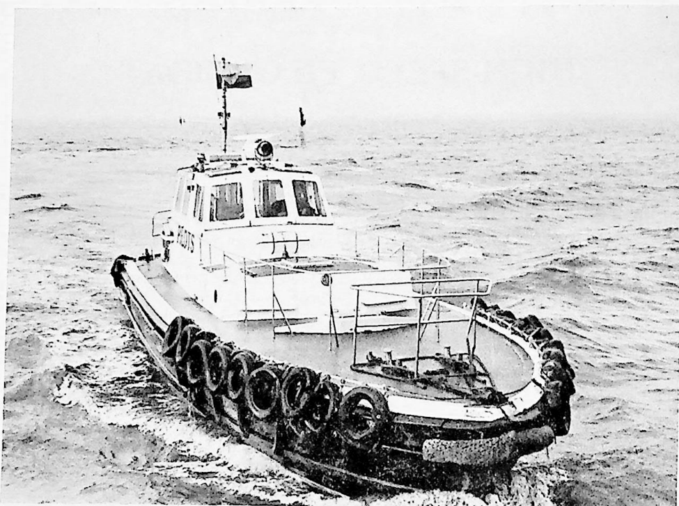
Captain J W Evenden, the GRP 50-footer, showing ample fendering and inboard handrails layout.
