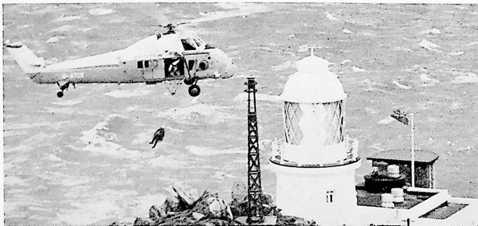
Recovering the winchman after slipping the cargo net at Lundy North. The flag and wave crests give some idea of the operating conditions.
