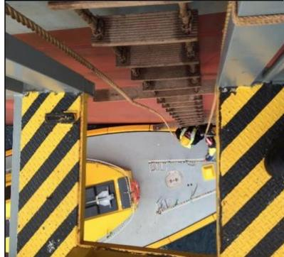
Recently a container vessel that arrived at the Port of London, the pilots were presented with a non-compliant trapdoor arrangement which they refused to board. The vessel remained at anchor as no suitable arrangement for safe boarding could be presented; the vessel sailed without berthing to its next port of call in Europe.
