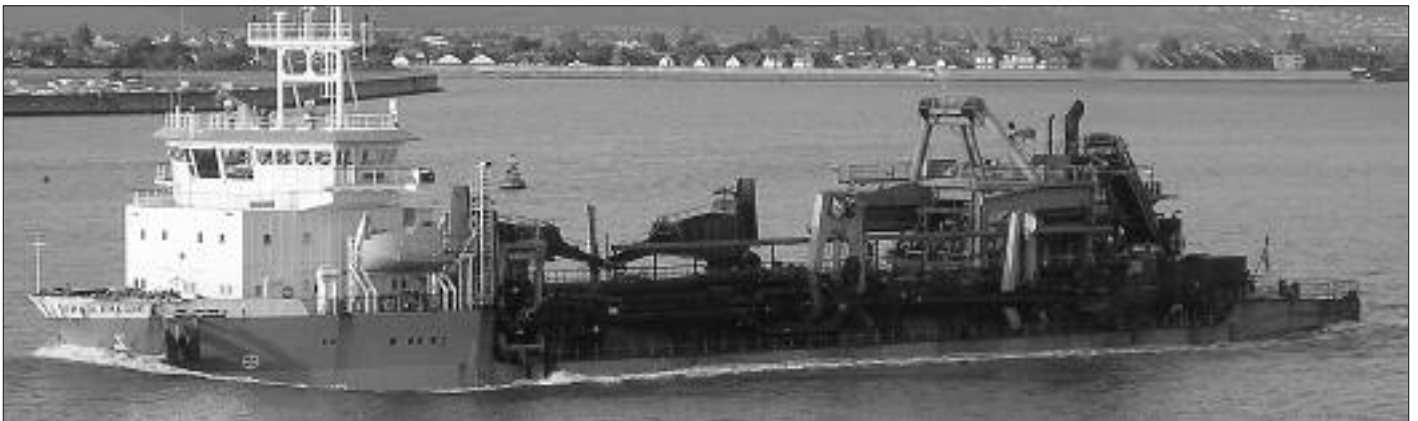
Ship speed 10kts. According to squat tables the deck should be submerged! Photo JCB
