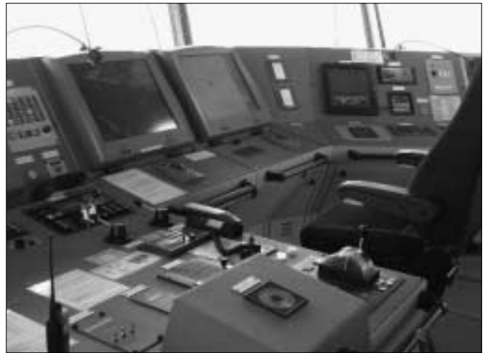
Picture 4: A good integrated bridge
