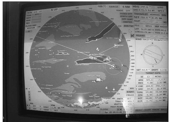
Picture 6. Radar with AIS and chart overlay
