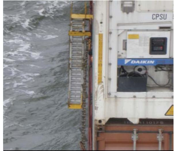
An example of the problems faced by pilots when ladders hang away from the ship's side
